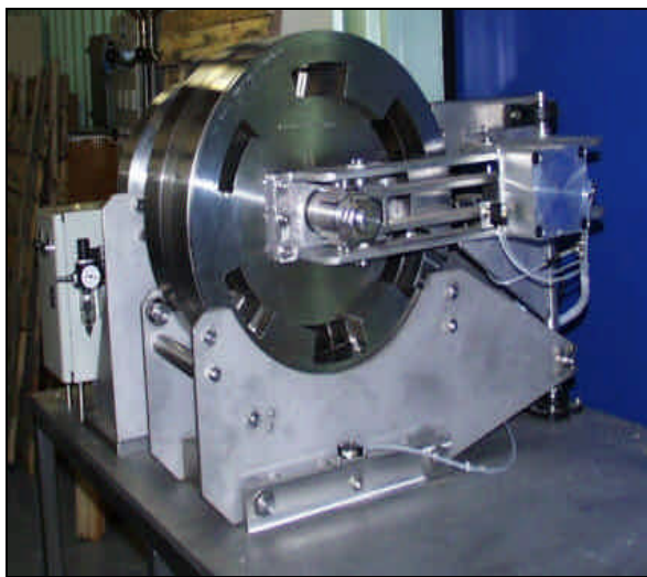
Figure 1 : CEA Prototype 10 litre rotating autoclave
