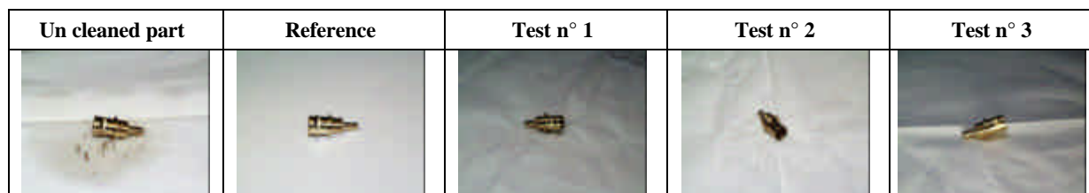
Figure 5 : SC CO 2 cleaned stainless steel alloy parts on white paper tests pictures
